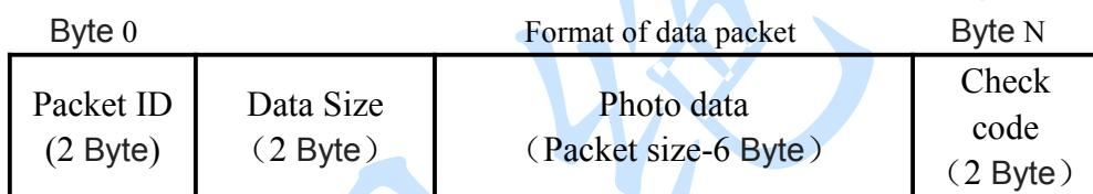
Packet ID: Serial number of packet, each photo data packet ID start from 0
